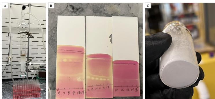
**Figure 3. A. Flash silica gel column chromatography set-up. B. Pure compound **1** (fractions 10 – 22). C. Compound **1****
