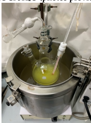
Figure 2. Reaction set-up for the diamination (photo provided by checkers)
