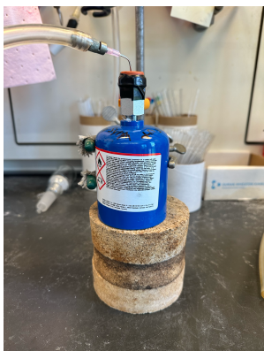
Figure 4. Properly secured bottle of DIBAL equipped with a taped septum. The headspace is under an inert gas atmosphere.
