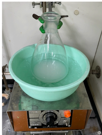
Figure 3. White Emulsion After the Addition of \text{Ca}(\text{OCl})_2 (photo provided by authors)
