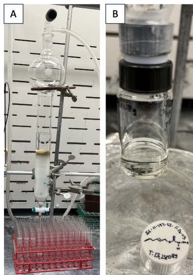
Figure 2. A. Flash silica gel column chromatography set-up; B. Pure product 1 (( E )-hex-2-en-1-yl methoxycarbamate) is a colorless oil
