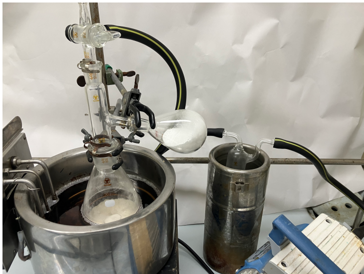
Figure 3. An apparatus of the drying process in which sodium trifluoromethanesulfinate is placed in the 300 mL flask. (The photo was provided by checkers)
