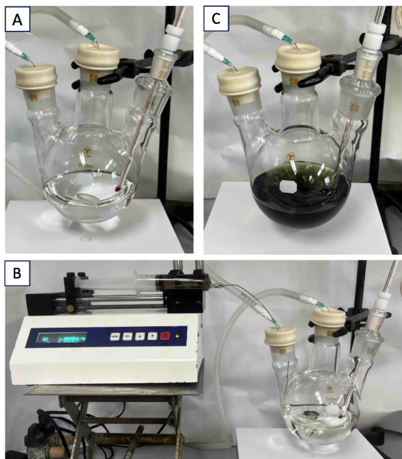
Figure 2. A. The reaction setup; B. The addition of the MeMgBr; C. The solution after the addition of MeMgBr (Photos provided by checkers)
