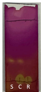
Figure 4. TLC of the crude reaction mixture after 14.5 h (S = methyl 3-bromopropionate, C = co-spot of S and R, and R = reaction mixture)
