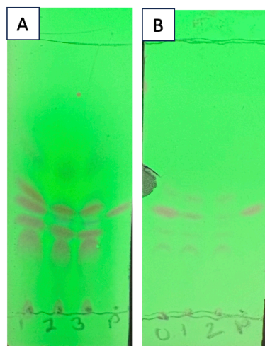
Figure 9: TLC of purified product (P, R_f = 0.46 ) versus organic layer after each set of 3 extractions. A. suspension of crude mixture in ethyl acetate; B. combined wash layers. After the extraction is complete, product is not detected in the organic layer
