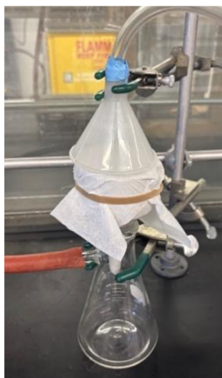
Figure 5. Setup for nitrogen sweep and vacuum drying of the crude product using a Büchner funnel fitted with a Kimwipe and rubber band
