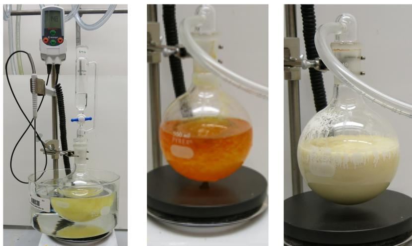
**Figure 1.** Reaction assembly for Step A before addition of  $\text{H}_2\text{O}_2$ , after addition of  $\text{H}_2\text{O}_2$ , and after mixture has stirred for 16 h
