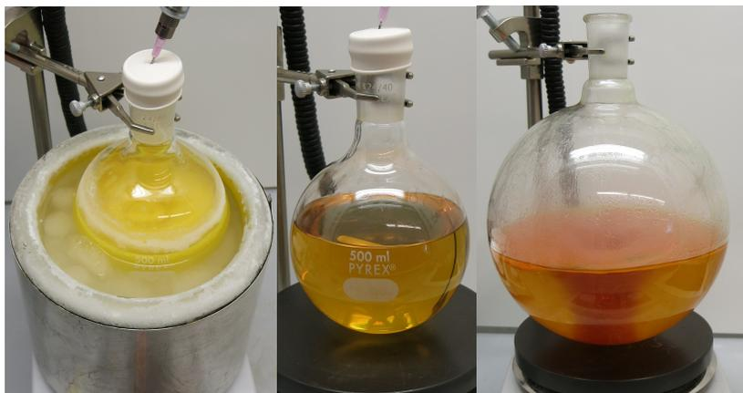
**Figure 3. Reaction assembly for Step B after the addition of *n*-BuLi, after addition of DMF, and after mixture is poured into aqueous HCl**
