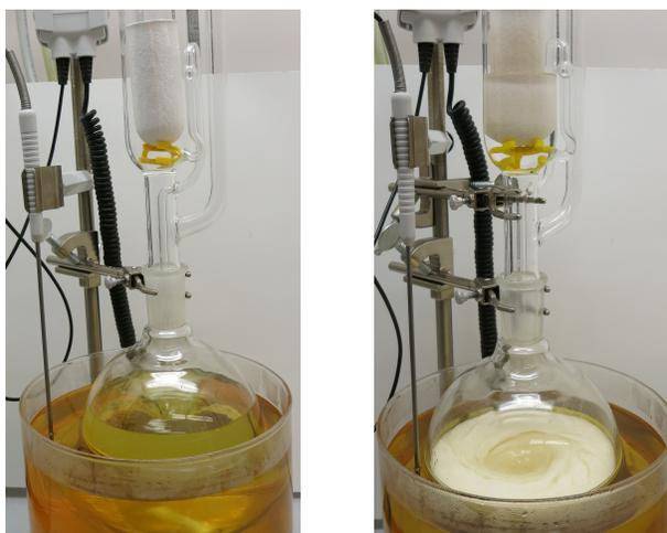
**Figure 2.** Soxhlet extraction assembly before extraction and after 48 h extraction.
