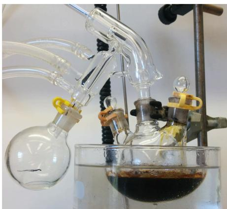
**Figure 6. Distillation Apparatus for Removal of Ethylene Glycol (provided by Checker)**
