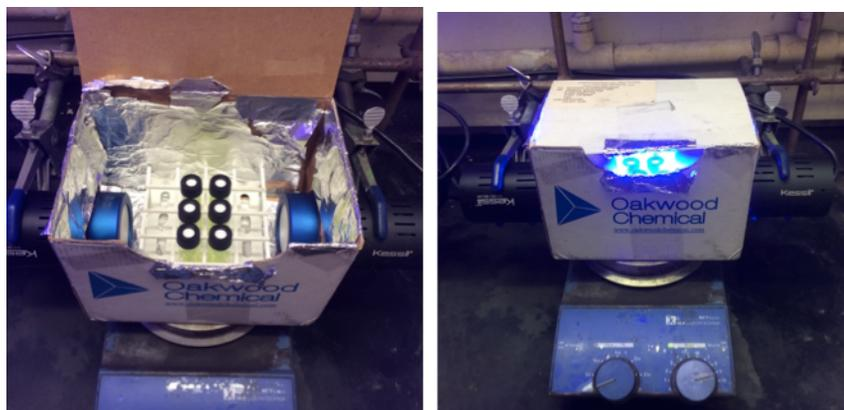
Figure 3. Visible light reaction set-up
