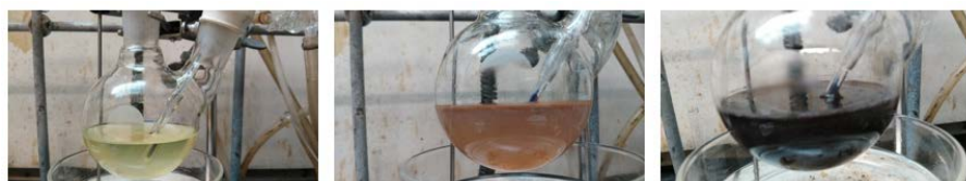
Figure 4. Progression of color from yellow to black in Step B
