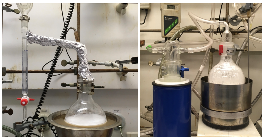
Figure 1: Step A - Dean-Stark trap and evaporation of remaining pivalic acid and water with a liquid nitrogen cold trap
