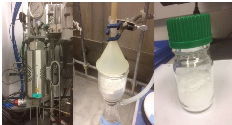
Figure 4. (A) Hydrogenation apparatus used in Step D; (B) \text{TMS}^{13}\text{CH}_2\text{NH}_2 \cdot \text{HCl} drying under nitrogen; (C) \text{TMS}^{13}\text{CH}_2\text{NH}_2 \cdot \text{HCl} product in a screw cap flask (photos provided by checkers)
