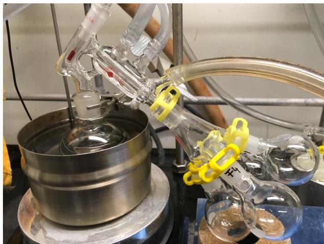
**Figure 2.** Distillation apparatus for the distillation of aryl ketone **2** (photo provided by submitter)
