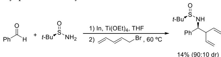
**Scheme 4. One-pot In-promoted pentadienylation of an in situ generated *N*-tert-butylsulfinyl imine**
