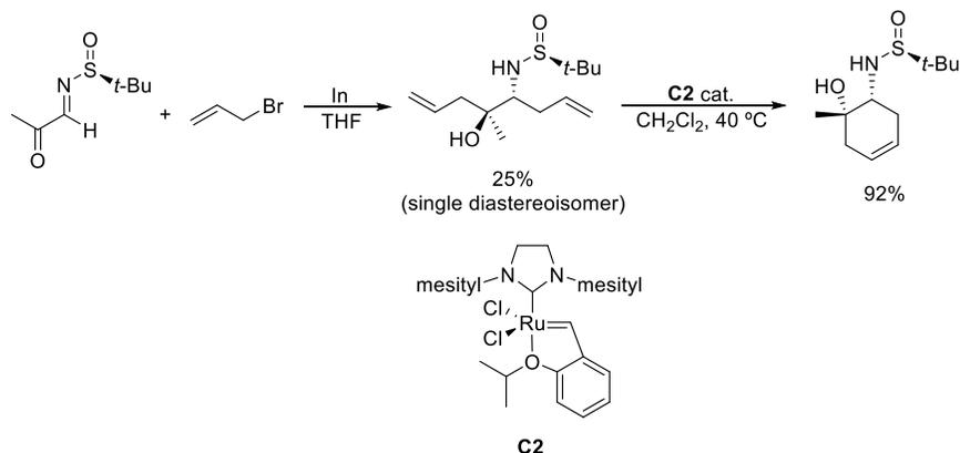
**Scheme 7. Diallylation of an  $\alpha$ -keto *N*-tert-butylsulfinyl imine and ring-closing metathesis**
