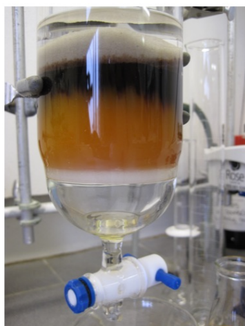
Figure 2. Filtration of the crude product on silica gel (left) and crystals of the major diastereomer (right, photos provided by submitters)
