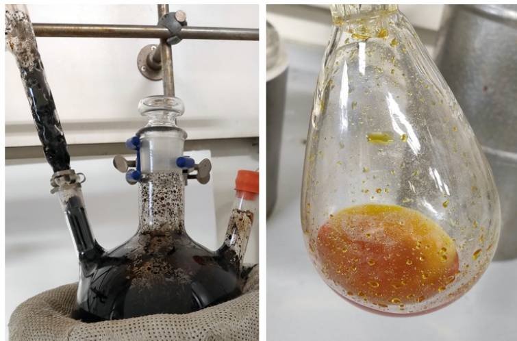
Figure 4. Appearance of the PEG and charred cellulose (left) and the distillate obtained (right)
