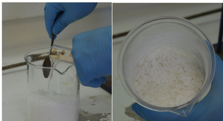
Figure 2. Diluted H 2 SO 4 being added to PEG (left) and appearance of the PEG/acid/cellulose mixture (right)
