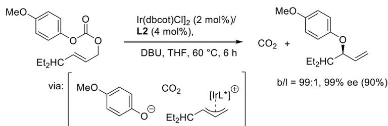
**Scheme 8. Tsuji-type decarboxylative allylic etherification**
