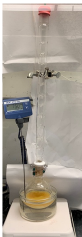
Figure 3. Full reaction setup with air condenser and nitrogen inlet needle (photo provided by submitters)
