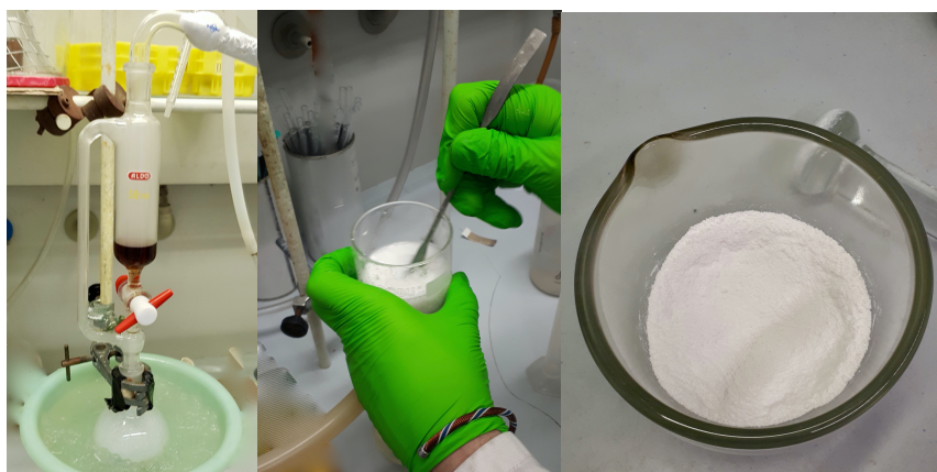
Figure 1. Addition set-up (left), trituration (middle) and final product (right) (photos provided by submitters)
