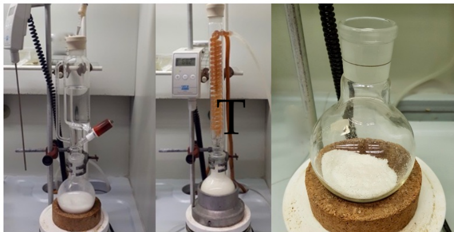
Figure 2. Reaction set-up (left), reflux set-up (middle) and final product (right) (photos provided by submitters)
