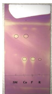
Figure 7. TLC of starting material (SM) versus reaction spot of the end of reaction (P), a central co-spot (Co) and a spot for the product (R). (photo provided by submitters)
