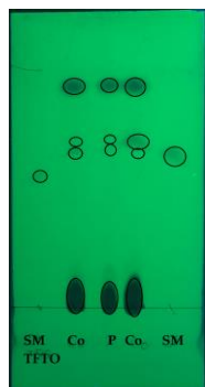
Figure 8. TLC of starting material tetrafluorothianthrene- S -oxide (SM TFTO, left) and starting material 2-phenylethyl acetate (SM, right) versus reaction spot of the end of reaction (P). A central co-spot (Co) for both is also shown (photo provided by submitters)
