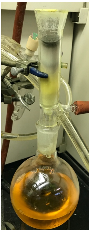
Figure 2. Filtration of 1 through silica gel (Photo provided by submitter)
