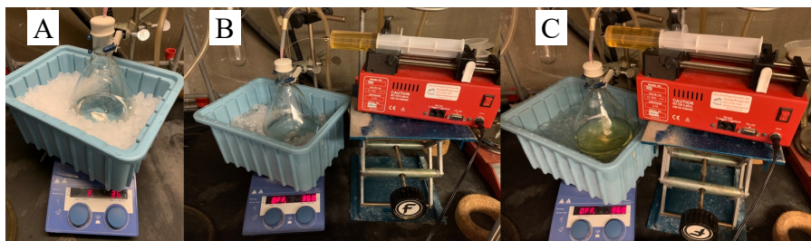
Figure 4. A) Reaction flask set-up after addition of starting material (1) and toluene; B) reaction solution before the n -BuLi addition; C) reaction solution during the n -BuLi addition (photo provided by submitter)
