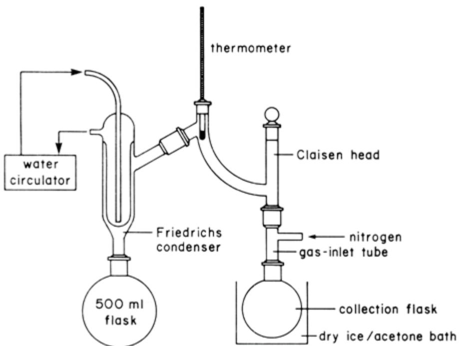
In the 250-mL flask is placed 100 mL of **dicyclopentadiene** (Note 1). The material is heated at reflux (bath temperature 200–210°C) under a **nitrogen** atmosphere (Note 2). After a 5-mL forerun is collected and discarded, the collection receiver is cooled to –78°C and 25 mL (0.30 mol) of **cyclopentadiene** is rapidly distilled at bp 36–42°C. A slight positive pressure of **nitrogen** is maintained throughout the distillation to prevent moisture from entering the system.
