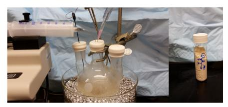
pump (Note 9). Upon complete addition, the mixture is stirred for an additional 4 h. The resulting slurry is allowed to cool to ambient temperature, concentrated by rotary evaporation (55 °C, 15 mmHg), crushed with a spatula, and further dried under high vacuum (< 12 mmHg, 12 h) to afford (S)-N-(1-chloro-3,3-dimethylbutan-2-yl)picolinamide hydrochloride salt as a tan powder (10.68–10.86 g, 38.5–39.2 mmol, 96–98% yield) (Note 10). This material is used without purification.
