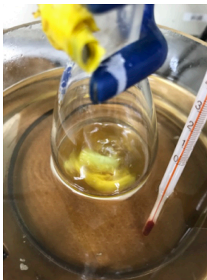
Figure 10. Reaction setup Step B (while heating at 130 °C)
