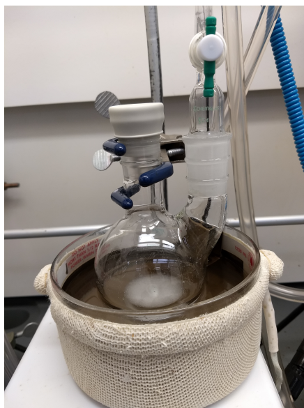
Figure 1. Reaction Setup for Step A (acetophenone oxime)
