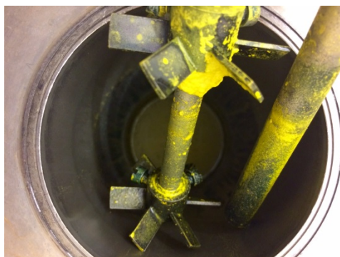
Figure 2. An example of the insoluble yellow solid found on the internal components after a successful reaction
