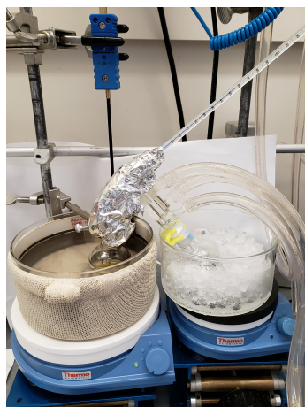
Figure 4. Distillation setup for purification of cyclopentylbenzene ( 2 )
