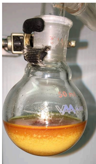
Figure 6. Precipitate formation 10 minutes after addition of the acetophenone
