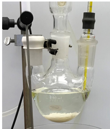
Figure 1. Experimental set-up and addition of (2 S ,3 R )-noscapine
