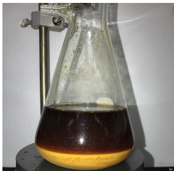
Figure 10. Precipitate crashing out of solution at pH 11 upon completion of reaction
