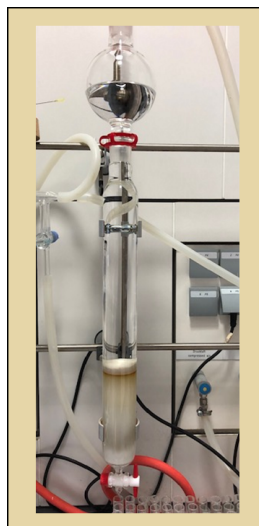
Figure 4. Glass column loaded with a slurry of silica, the crude product, and sea sand, eluted with ethyl acetate and hexane (photo provided by submitters)
