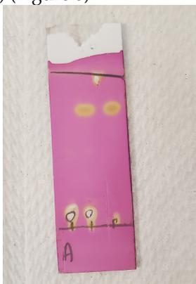
**Figure 6.** The reaction progress at 18 h visualized by  $\text{KMnO}_4$  stain. To TLC 2, a drop of the reaction solution was removed and diluted with 0.5 mL of DCM. A = 1 and the third lane contains the reaction.
