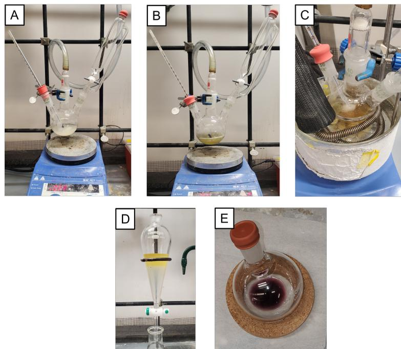
**Figure 3. A. The reaction color at the start of the reaction; B. The reaction color after 2 hr; C. The color of the reaction after the addition of the butenolide 2; D. The aqueous and organic phases in the separatory funnel; E. The crude purple oil**
