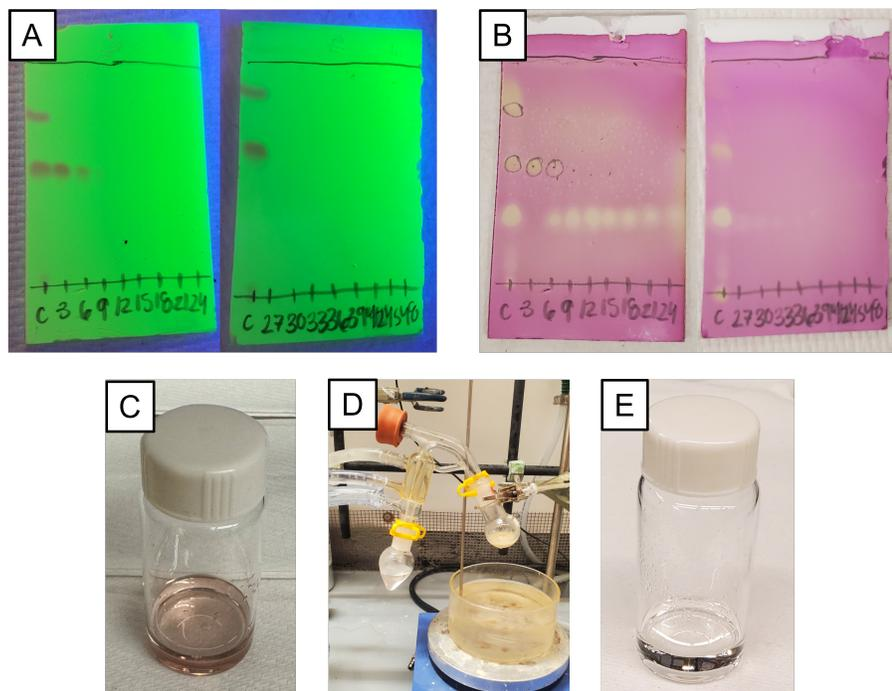
**Figure 4.** A. TLCs from column chromatography visualized using UV (254 nm). Fractions 6-39 were combined ( $R_f = 0.4$ , 4:1 hexanes:EtOAc); B. TLC of the fractions stained with  $\text{KMnO}_4$  stain; C. Resulting purple oil of the combined fractions; D. The distillation set up after completion of the distillation; E. The pure material as a clear oil
