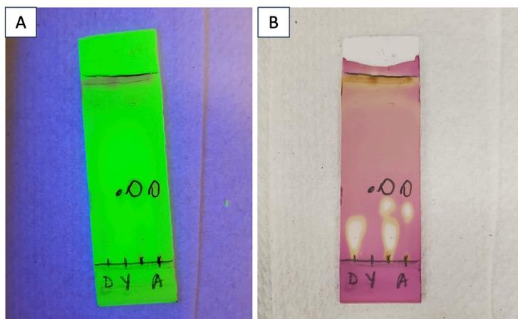
**Figure 5. A. The reaction progress at 18hrs under UV (254 nm). To TLC 1, a drop of the reaction solution was removed and diluted with 0.5 mL of DCM. D = 1,3-dihydroxyacetone, Y = (carbethoxymethylene) triphenylphosphorane, A = product. The circles in pencil correspond to UV active spots; B. The reaction progress at 18 h in  $\text{KMnO}_4$  stain**
