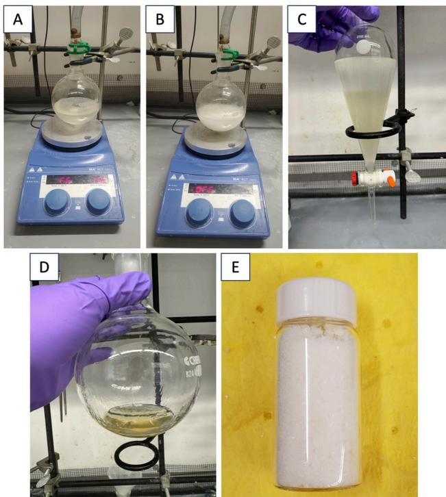
**Figure 2.** A. The reaction color after the addition of imidazole; B. The reaction cloudiness after the addition of TBSCl; C. The aqueous and organic phases in the separatory funnel; D. The crude yellow oil after concentration; E. The final product obtained as a white solid after recrystallization
