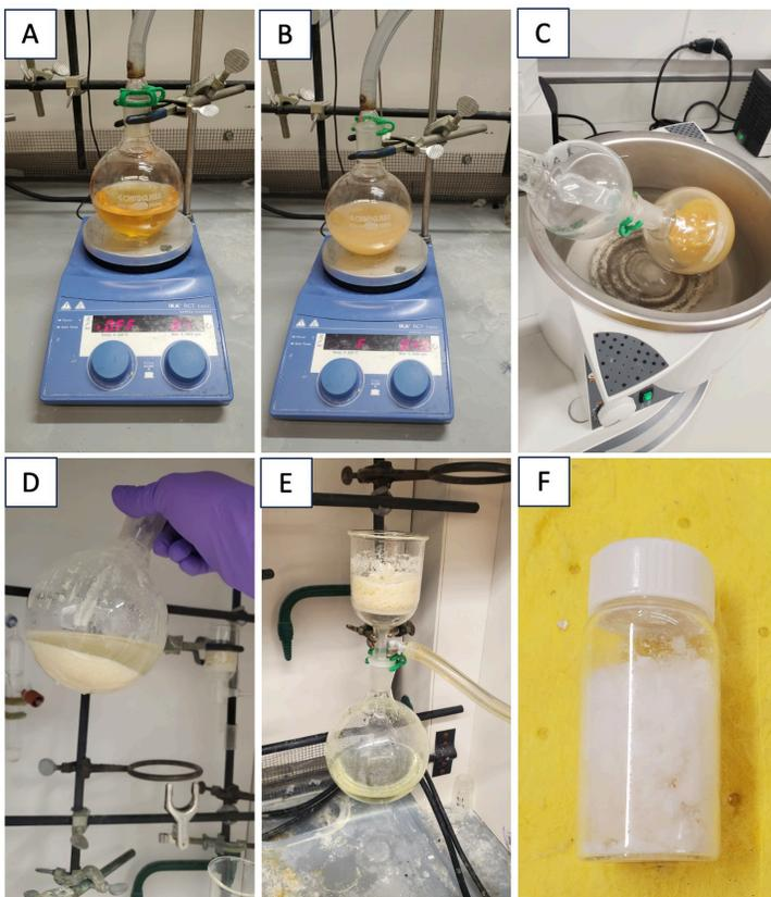
**Figure 1. A. The reaction color and turbidity at the beginning of the reaction; B. The reaction color and transparency at the end of the reaction; C. The color and consistency of the concentrated reaction; D. The precipitated TPPO byproduct after sonication; E. The filtration of the TPPO byproduct and pale-yellow aqueous filtrate; F. The final product obtained as an off-white powder**
