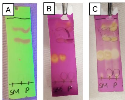
**Figure 7. A. The reaction progress at 3hrs in under UV (254 nm). The crude 3hr NMR sample was used as a TLC sample for 3 (P). SM = 2. The circles in pencil correspond to UV active spots; B. The TLC after immediate exposure to  $\text{KMnO}_4$  stain; C. The TLC after development of the  $\text{KMnO}_4$  stain**
