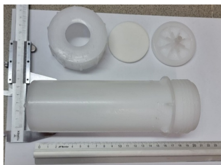
Figure 10. An empty flash chromatography cartridge used for purification of product 3
