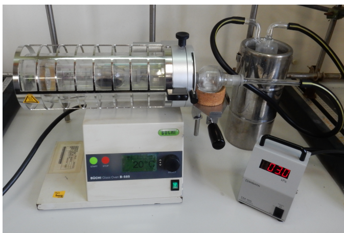
Figure 3. Distillation set-up using a Kugelrohr apparatus
