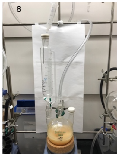
Figure 8. Rinse of residual solid with dichloromethane using a syringe (provided by checker); Figure 9. Reaction flask with final reaction mixture before extended stirring. (provided by checker)
