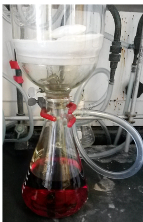
Figure 12. Salts removal by filtration through a sintered glass funnel over a pad of Celite
