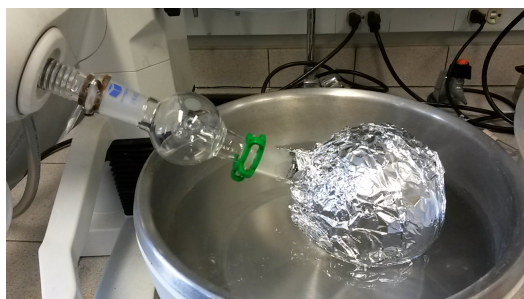
Figure 13. Light protection with aluminum foil for evaporation
