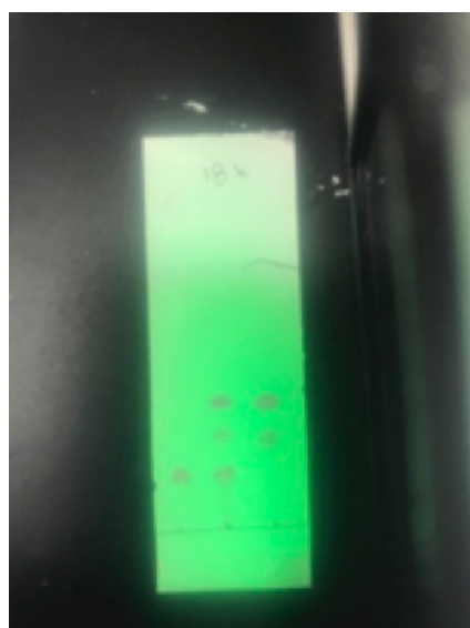
Figure 5. TLC analysis of Step A reaction progress at 18 h: Left lane = ( R )-BINOL; Right lane = reaction mixture; Middle lane = cospot. Top spot in right lane corresponds to desired product, bottom spot corresponds to mono-methoxymethyl protected BINOL
